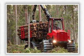
Forwarders are articulated forest machines whose main build features include the presence of a hydraulic crane and a height adjustable bunk structure which allows collecting and hauling fully suspended the whole round wood from thinnings and final cuttings.
