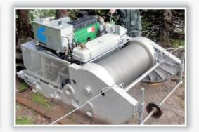
The skyline is a cable stationary installation with a sledge winch and a carriage and it is used in forest exploitation for retrieving and gathering the wooden mass from rough terrains, on medium and long distances from both thinnings and final fellings.
