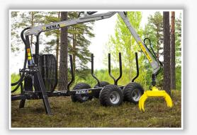
Forestry trailers are equipped with a hydraulic crane for loading and unloading the round wood. They represent a cheaper alternative to the forwarder, especially in the hill areas of forest exploitation, where the slopes are moderate or in areas with young trees, where access with heavy equipment is harder.
