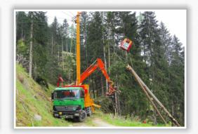
The yarder is a mobile skyline installation with the driving unit fitted on the tractor, forestry truck chassis, trailer chassis or tracked chassis. Its main feature is the folding, telescopic (optional) mast which provides adequate height for the cables in the initial point of the line.
