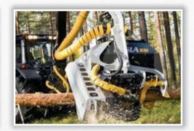
This hydro-mechanic equipment is attached to specialized harvesting forestry machines, excavators both with wheels and on tracks and are operated by an electronic computer. It fulfills all the processes of harvesting the wooden mass from cutting to delimbing, debarking and cutting the logs to size.
