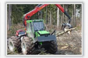
Skidders are specialized forestry machines, suited for hauling long trunks from thinnings and final fellings. They're equipped with a frontal blade, double-drum winches with different traction forces and optionally, for light terrain conditions, with a hydraulic crane, for suspending one end of the round wood on the back shield and stacking the logs on landing sites.
