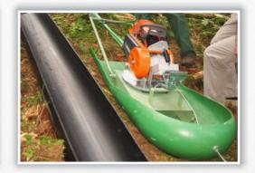
Log lines are slope skidding installations utilized in the ecological gathering of the wooden mass from thinnings on steep slopes. With the aid of this technology wood gathering is done without harming other standing trees or the soil, its flexibility giving multiple ways of avoiding any obstacles.
