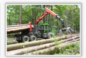
Combi machines are articulated forestry tractors with a 6wd or 8wd transmission, which can be found in technological fluxes of every kind, regardless of the type of cutting involved (thinnings or final fellings).
