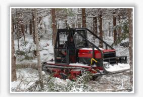
The mini-skidder is a tracked skidder used primarily in thinnings.
